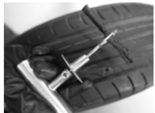
9. Thread a single repair plug through the eye in the end of the inserting tool until there are equal lengths of the plug on either side of the tool.
