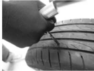
5. Push the reaming tool into the punctured area, push in and out while rotating left and right to make a hole big enough.
