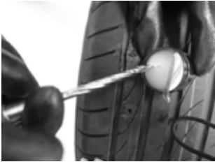
4. Apply the lubricant supplied to the spiral hole reaming tool.
