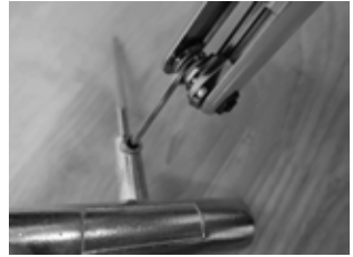
6. Replace the round file and tighten it with 3mm hex key.
