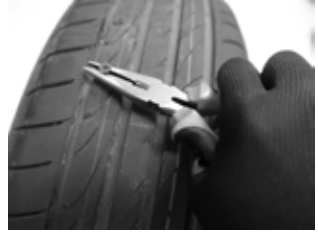
3. Remove object that caused the puncture with pliers.
