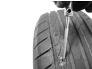
7. Push the round file into the punctured area, push in and out while rotating left and right to make a hole big enough for a repair plug to be inserted.
