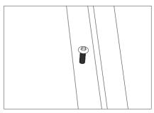
+ Position the Camp Kitchen X-Lite on the flat surface. Use the 6 x M6 bolts to fix on the surface.
