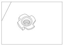
+ Flatten the Tee Nuts with a mallet or hammer.
