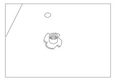
+ Insert the Tee Nuts into the holes ensuring the nuts are upright and square to the hole.
