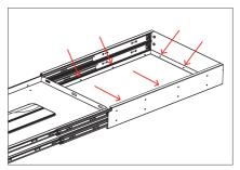
+ Mark the six drilling points through the fixing holes with a permanent marker.
