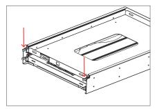
+ Pull out both fridge slide and stove top by pressing the lock levers on both sides, then fully pull out to reveal the fixing holes on the side rails.
