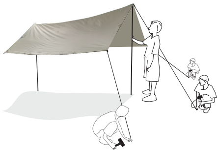
Pole into the other end of the grommet, One person holds the pole, while the other nails the drawstring at 3
