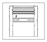
+ To access the bottom mounting rail,loosen the screws on the top panel and carefully remove the top panel. Then gently pull out the drawer tub. After assembly make sure the top panel is screwed back firmly into place.
