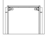
+ Release the two latches at rear of drawer for ease of removal.
