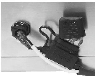
15A Replaceable inline fuse protection
