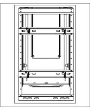
Pull out the slide to allow easy access bottom mounting rail.Using the M10 bolts and nuts/washers provided in the mounting kit to attach to the underside of the camp kitchen.
