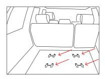
You can use the seat anchor points to bolt the camp kitchen into your car. Check the distance between the seat mounting points and compare with the mounting rail at bottom of camp kitchen.
