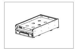
+ The top section of the slide is designed placement of your fridge/freezer. Using the four straps supplied, loop them through the oval holes at each end to hold the fridge firmly in place.
