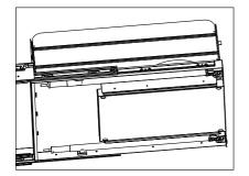
+ Support legs are underneath the third section of the slide.
