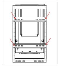
+ Move the mounting rail to adjust to right position.
