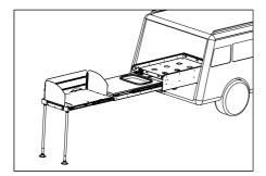
+ The third section of the slide is where you place your stove. To set up the wind shield, you will need to release the wind shield from the bungee cord and clip into the slots provided.
