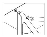
Step 2: Lift the body frame up to assemble the rear cross rib by using M6x12mm bolts (9) and M6 Nyloc nuts (10).
