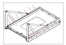
+ Mark six drilling points through any of the 14 fixing holes with a permanent marker.
