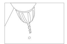
+ Drill six 7mm holes for the Tee Nuts.
