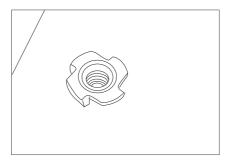
+ Flatten the Tee Nuts (2) with a mallet or hammer.
