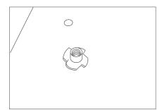
+ Insert the Tee Nuts (2) into the holes ensuring the nuts are upright and square to the hole.
