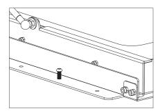
+ Position the fridge slide on the flat surface. Use the 6pcs M6x20mm bolts (1), M6 washers (13) and M6 Nyloc nuts (4) to fix to the surface.
