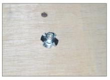
+ Insert the Tee Nuts into the holes ensuring the nuts are upright and square to the hole.
