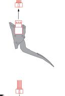
unit in-line between the factory plug and pedal assembly. Ensure the plugs are aligned correctly to prevent damage to the internal pins. Locate a suitable position on the dash or console for the evcX driver interface. Be aware that the LED display is bright and should be positioned so as not to
