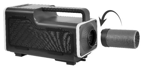
3. Remove the end cap from the drain hole. Insert the drain pipe into the drain hole at the back of the air conditioner. Keep the drain pipe straight to avoid clogging.
