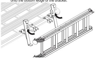
The ladder is slid up under the top hook of the bracket, then comes to rest on the lower ledge.
