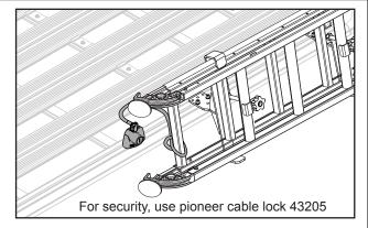
The brackets will swing out of the way, releasing the ladder.
