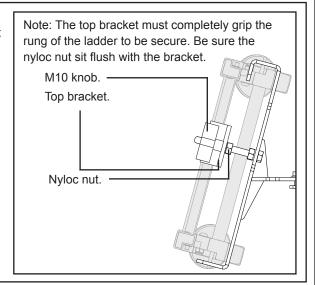
To remove ladder, loosen M10 knob and swing the brackets down as shown.
