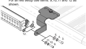
Fix the Light Bar to the Brackets using the hardware supplied within the Light Bar Kit purchased.
