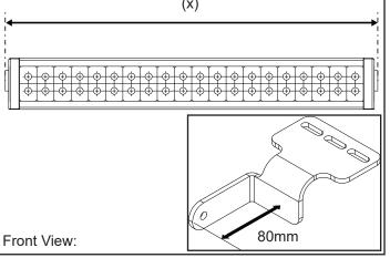
Attach the Brackets onto the Platform by first sliding an M8 Channel nut into the 'C' channel of the Platform. Place the bracket over this and fix in place with an M8 Button Head Screw, M8 Spring and Flat
