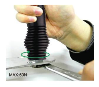
3. Remove the cap from the top of the spring base and install the fiberglass extension pole on to the base by turning in a clockwise direction and secure in place with the grub screw (using the hex key provied). Hand tighten only MAX. 15N.
