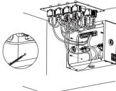
Lift the control box onto desired location, mark the locations of the drilled mounting holes on the canopy wall. Remove the box and drill the holes accordingly.
