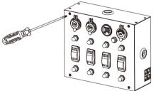
Unscrew the 4x flat head screws to open the cover plate by a hand screwdriver (not included). After opening the cover plate, make sure all wiring is properly connected and no internal terminal studs are loose.
