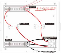
+ Once complete, the LED display on the voltmeter should be an indication of power going into the panel. If there is no power, check cabling, wiring, test using a 12v multimeter, or contact a licensed auto electrician.
