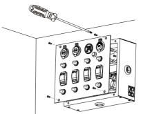
4.Fasten the 4x flat head screws by hand screwdriver (not included) to close the cover plate. Do not over fasten the mounting screws.
