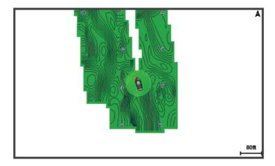
A green circle indicates good depth and GPS position, and a speed under 16 km/h (10 mph). A yellow circle indicates good depth and GPS position, and a speed between 16 and 32 km/h (10 and 20 mph). A red circle indicates poor depth or GPS position, and a speed above 32 km/h (20 mph).
