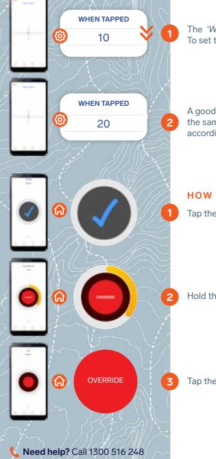
The *'When Tapped'* value controls the manual override brake response. To set the value, select *'When Tapped'* under Override in program screen.
