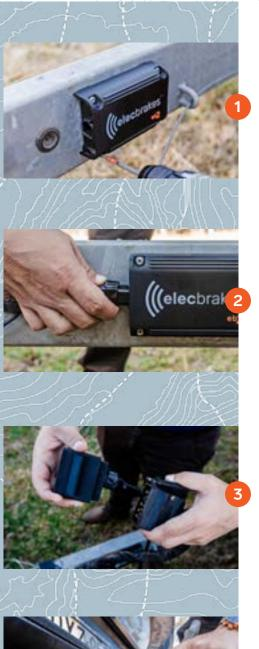
Fasten the unit to the draw bar using the mounting screws provided.
