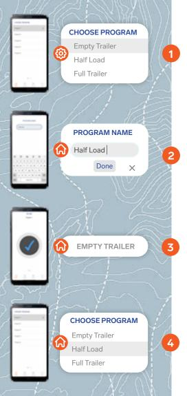
You must be connected to the brake controller to set and activate programs. Navigate to the '*Settings*' page and select a program.
