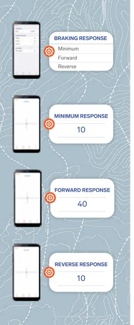
Your EB2 unit comes with default brake settings. We recommend adjusting your brake response to your specific requirements. To adjust the **minimum**, **forward** and **reverse** response, tap 'settings' on the app.
